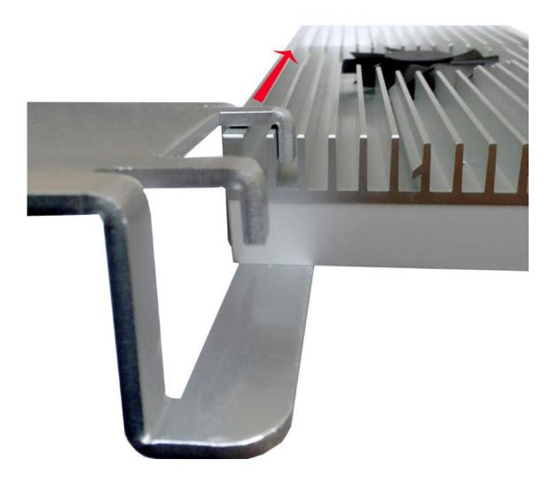
3. As the bracket approaches the control button on the back of the light unit lift the bracket away from the button slightly to avoid damaging the status control button.
