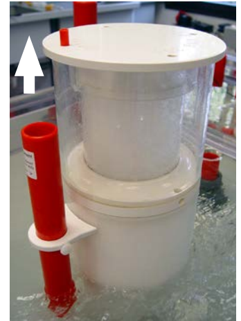
Nozzle with air- and ozon- plug
