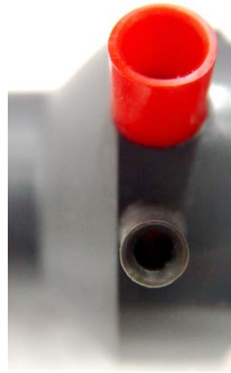
Nozzle with air- and ozon- plug
